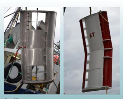
**Figure 5.7:** 2 m<sup>2</sup> (left) and 9 m<sup>2</sup> (right) trawl doors equipped with hatches, which are used to adjust depth and horizontal spread.
