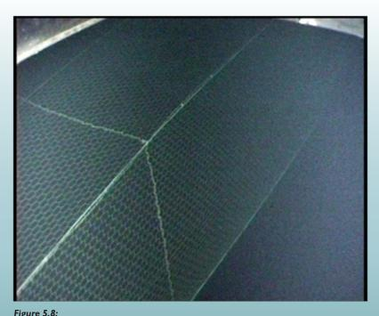
Aft trawl belly made from brick-shaped meshes.
