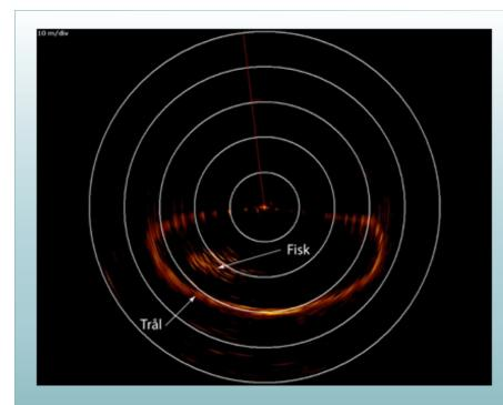
*Figure 5.3:* Sonar picture of the trawl mouth and entering fish.
