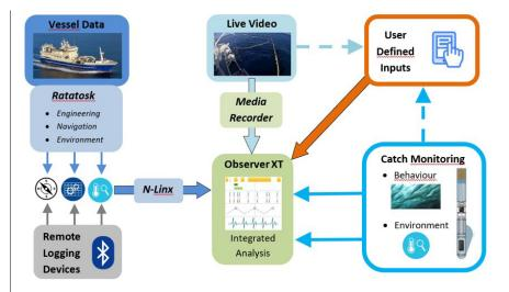
Figure 5.2.5. An overview of the compilation and integration of data (behavioural, engineering, environmental, and navigational) from several sources (vessel, live video, remote logging devices, catch monitoring devices and user defined inputs) via the Ratatosk, N-Linx, Media Recorder and Observer XT systems (Source: Catch Control in Purse Seine - https://www.sintef.no/projectweb/fangstkontroll/).
