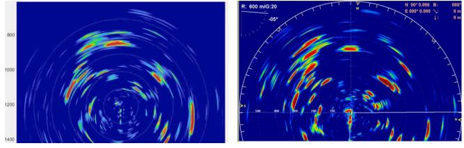
Figure 5.2.2. Display of sonar raw data processed with new developed algorithms (left panel) and screen dump from the sonar display from Simrad SU90 for the same second (right panel).
