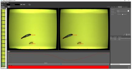
Figure 5.3.9. Example Deep Vision image from 800 m depth during an IMR mesopelagic cruise. Upper object is a glacier lantern fish (Benthosema glaciale), with length of 66 mm, lower object is a squid measured at 52 mm mantle length. Image Shale Rosen
