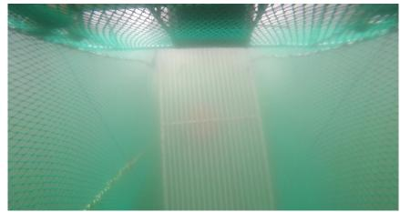
Figure 5.3.6. Prototype sorting mechanism. Håvard Vagstøl (Scantrol Deep Vision) adjusts motor before system is loaded on board FV "Fangst" for testing (left). Opening to release fish is visible in lower right corner of image. Sorting mechanism in "capture" position (upper right) and "release" position (lower right). Photos Liz Kvalvik.
