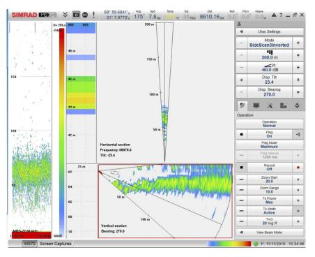
Figure 5.1.3. Measuring herring close to the sea surface with the MS70 sonar.
