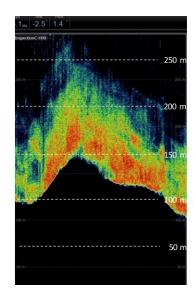
Figure 5.2.1. Vertical section of a capelin school using SN90 sonar with the closer edge of the school at 100 m at a depth of 20 m (left panel). An inspection beam oriented perpendicular to the school, show the decrease (from red to light green colour) in the acoustic backscattering from the closer part of the school at about 100 m towards the distant border about 170 m from the vessel. The range indicates, horizontal distance from the vessel (right panel).
