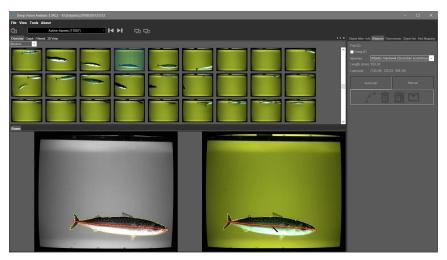
Figure 5.3.2. Example of automatic segmentation, object matching in left and right images, and calculation of length. In this example, the midline of the selected Atlantic mackerel (Scomber scombrus) is generated as a series of 25 segments, with a total length of 350 mm. Image courtesy Girona Vision Research SL.
