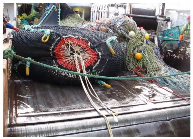
Figure 5.5.4. A catch in the dual sequential codend (left), and in the conventional codend (right).
