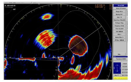
Figure 5.1.1. Dense capelin school where acoustic extinction occur, but not clearly shown in the sonar display. The catch was three times as large as first estimated.
