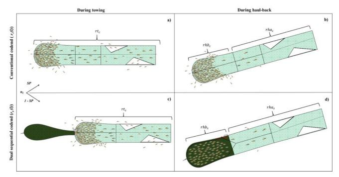
Figure 5.5.2. Schematics showing the size selectivity that occurs with the conventional codend (rc(l)) during (a) towing and (b) haul-back. (c) Size selection in the anterior codend segment of the dual sequential codend during towing, which, due to the codend design, (d) should cease during haul-back when the fish enter the posterior quality-improving codend segment. (The sections are not scaled according to each other).
