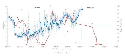
Figure 5.2.4. oxygen concentrations can become very low in the catch during pumping because of high crowding densities, which can significantly affect the "vitality" of the fish as they are pumped on board.
