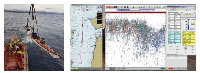
Figure 5.1.2. KayakDrone used on herring layers in Kvænangen, showing the echogram recorded onboard the Drone while passed by RV "G.O.Sars". The herring reaction to the research vessel was obvious as they started diving 100 meters in front of the vessel. Comparisons between densities measured from the vessel, from a drifting buoy, from the Drone and from the side-looking MS70 system will be made on this dataset.
