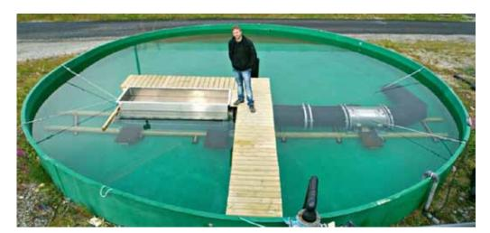
Figure 5.12. The CRISP large-scale swim tunnel was established in an 11 meter diameter outdoor tank at the Tromsø Aquaculture Research Station. Photo by Jon Are Berg Jacobsen (Nofima).
