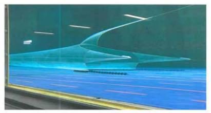
Figure 5.11. A bottom trawl equipped with an upper tongue to be lifted with the net-sounder cable when towed with a semipelagic rigging.
