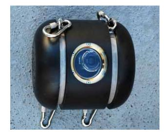
Figure 5.5. Observation unit for use during purse seine fishing. An underwater camera is mounted in a steel frame surrounded by a polyethylene protection unit.
