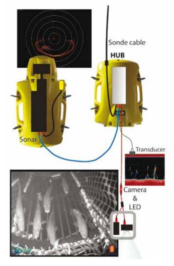
Figure 5.3. A system for observing fish and trawl behaviour by sonar, camera and echosounders.
