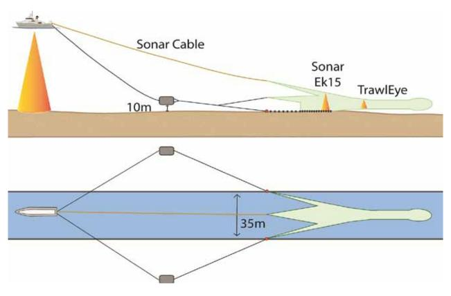
Figure 5.10. Rigging of the semipelagic trawl with the doors 10 m above seabed.
