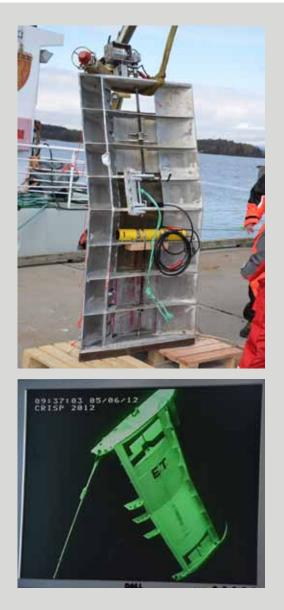
Figure 5.9. 2 m<sup>2</sup> (upper picture) and 9 m<sup>2</sup> (lower picture) trawl doors equipped with hatches, which are used to adjust depth and horizontal spread.
