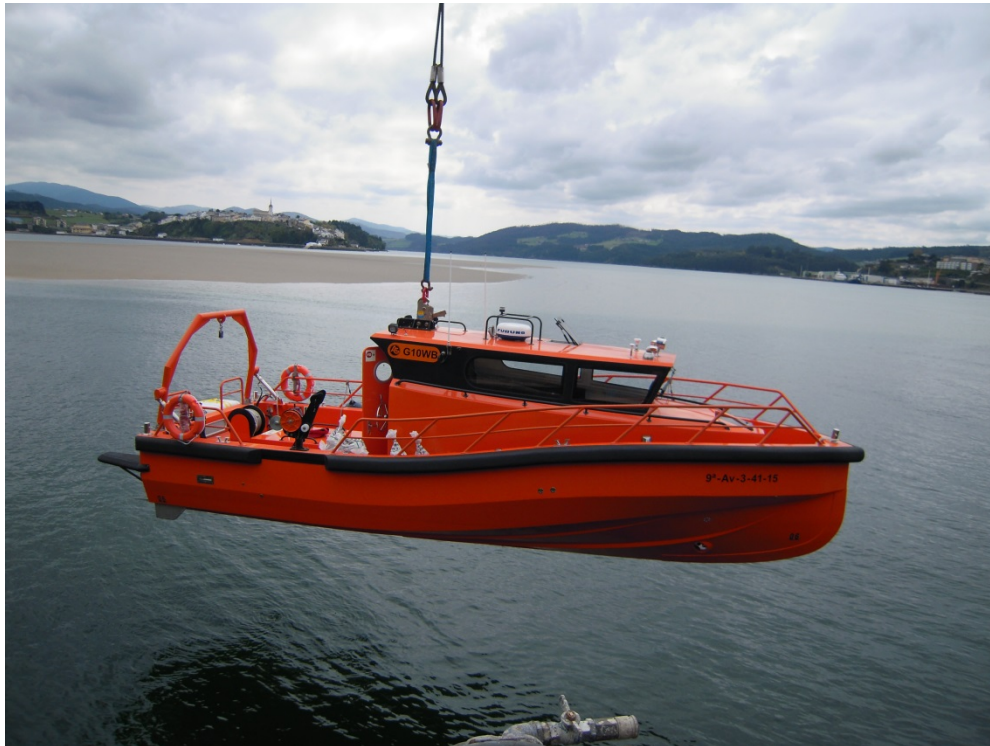
Work boat weight test
